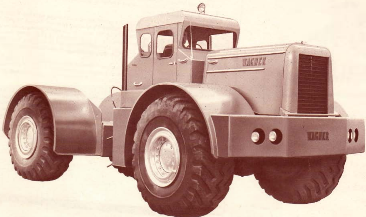
WAGNER TRACTOR MODEL 24 — 300 H.P. DIESEL POWER OTHER MODELS RANGE FROM 110 H.P. TO 600 H.P.
